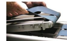
Quick release conveyors for ease of cleaning and replacement
